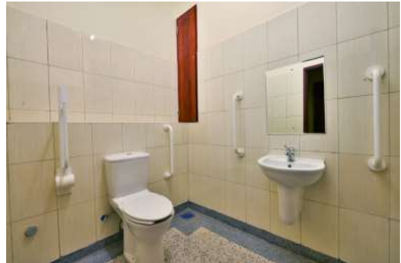
Toilet for people with disabilities
